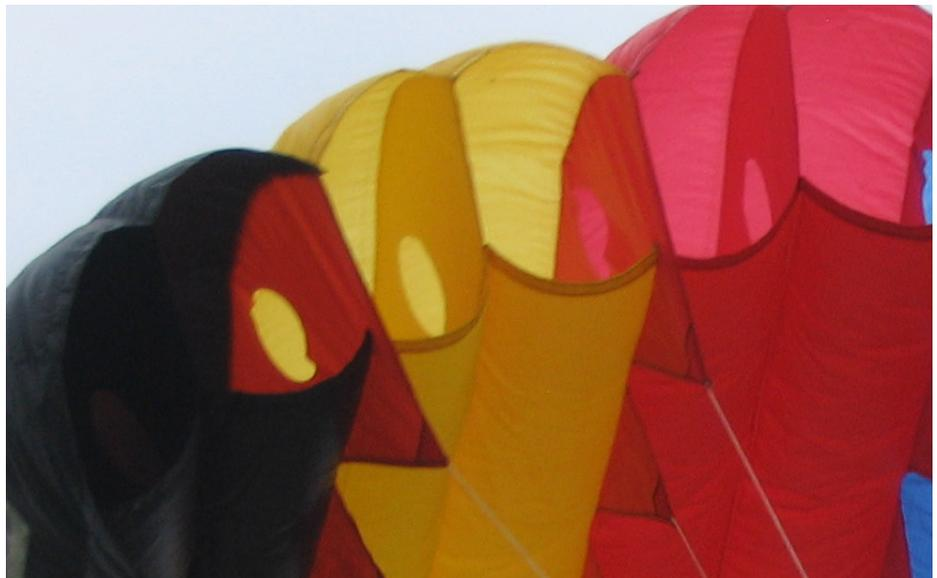
**In this close-up of a modern ram-air canopy you can clearly see the open leading edge, some crossports and flares. The open „mouth“ lets ram-air get into the cells in order to inflate them. The crossports help to maintain equal pressure in all the cells and keep end cells open. The flares improve directional stability and help to spread the stress imposed by the payload.**
