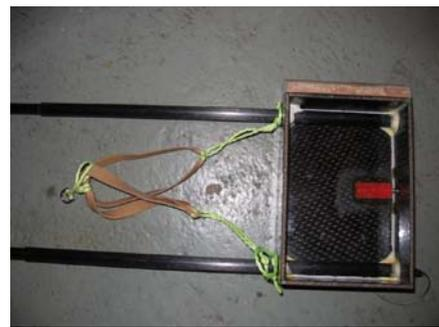
This jump box is made of carbon fibre. Of course 2 mm birch plywood would be sufficient too.
