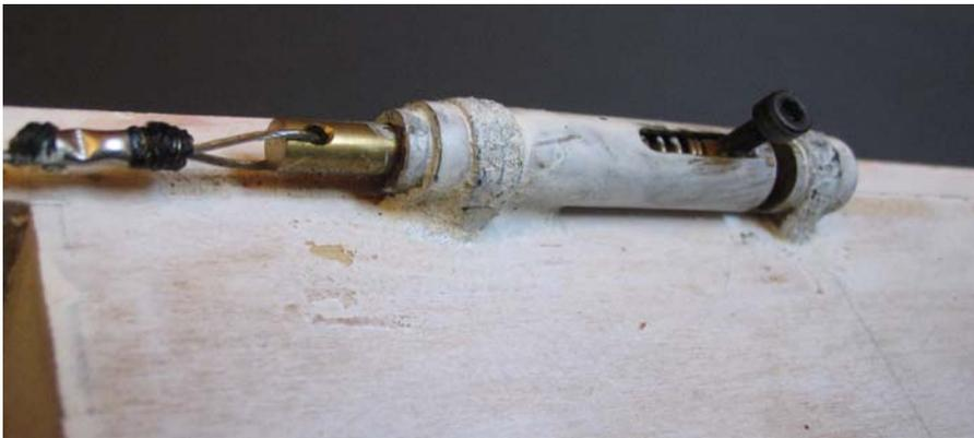
**This release mechanism is made of different sizes of brass tube, a spring and a piece of steel cable. The Allen screw is the „handle“ of the lock. The slot to the right of the screw takes the split ring. The steel cable retracts the „pin“.**
