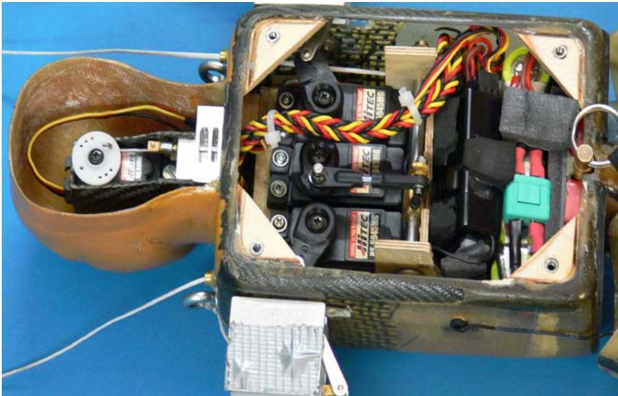
This MIKE is crammed with equipment. The release servo had to give way to the „block and pulley“ servo, which is the Hitec 5945 in the middle. In the middle you can also see the pushrod that moves the 5 mm silver steel shaft. The flanges are on the sides of the servo bay, which is made from 2 mm plywood.
