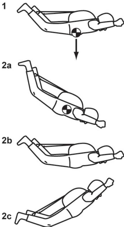
**1:** If the centre of gravity is in its correct position, the jumper stays in a stable horizontal position during free fall.
