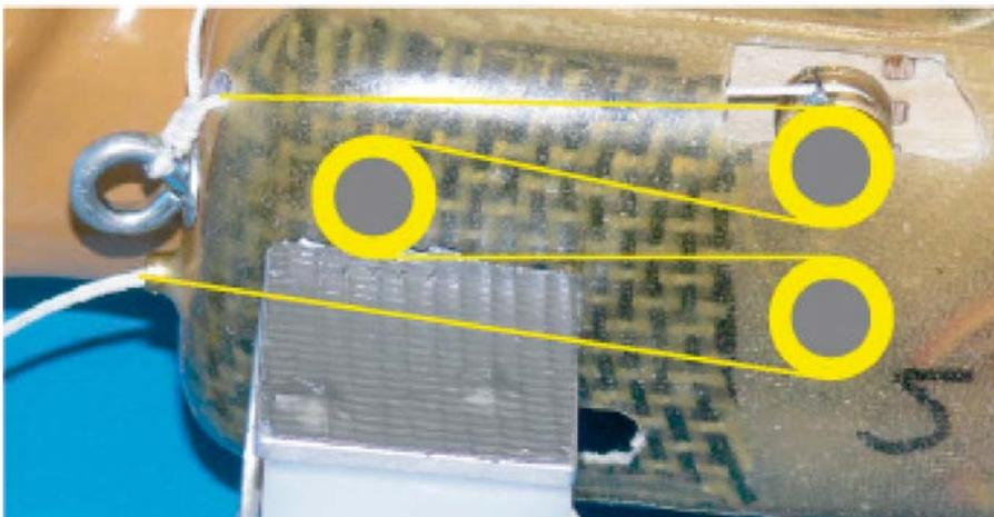
This picture gives you an idea on how the steering line is run through the mechanism.
