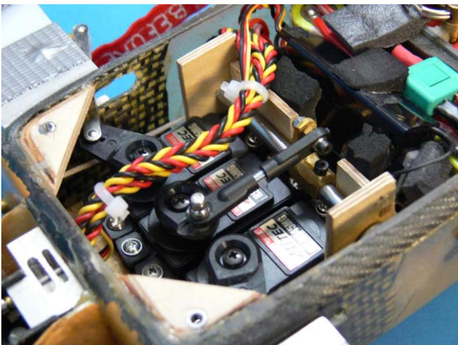
In this close-up you can clearly see the brass lever that operates the shaft.
