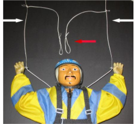
The white arrows highlight the main steering lines. The red arrow points out the interlaced lines used for deployment braking.
