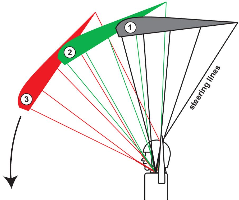
**To be on the safe side, we normally must deploy our parachute with the brakes set to a certain extent. A non-braked parachute immediately starts to move forward and downward once its fully open.**
