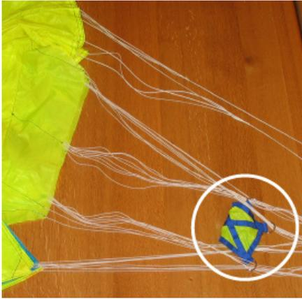
**Sliders can help to slow down the unfolding process of a canopy.**
