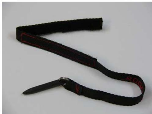
One of the „static-lines“ commonly used in Germany. The carbon pin is very lightweight and doesn't damage the fuselage.
